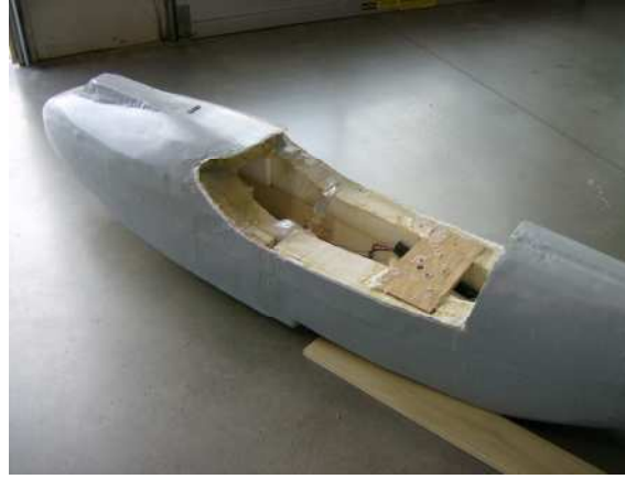
Construction is a lot of foam and fiberglass
